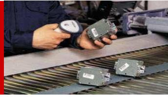
Manufacturers can track and record in-process assembly information into the RFID tag as an item progresses along the line. For example, as features are added to a personal computer assembly, they could be recorded on the tag. In this case, the tag would keep a current "inventory" of the PC's contents. The tag information could later be read to produce a shipping list and invoice. The tag could also remain with the item for later use by field personnel during installation and maintenance.
